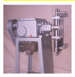
Unit comprises of an accurate Reciprocating Plunger Pump driven through an AC motor.
